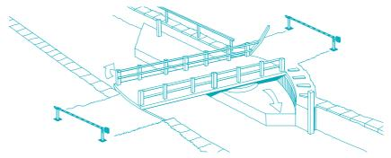
Unhook the retaining chain and give the bridge a good – but controlled – shove. You might need to slow the swing down to stop the bridge bouncing back across the canal when it hits the buffer stop.
