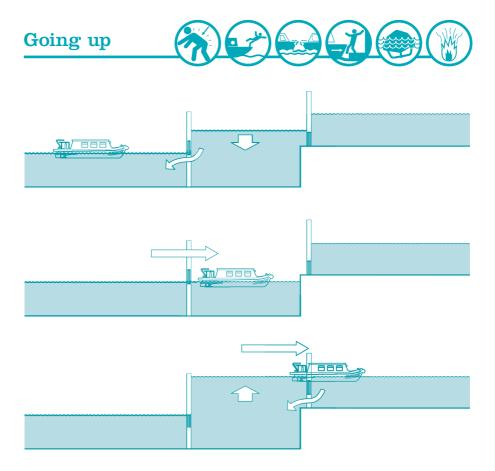
In wide and river locks keep your boat steady using front and back ropes looped round the bollards – take an extra turn around the bollard to stop the boat pulling you, but don't tie up.
