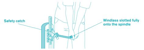
With one crew member at the helm and one at the paddles, you wind the paddle gear up and down using a windlass or lock key. You should always wind them bit-by-bit – and keep an eye on the effect of the moving water on your boat.
