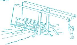
Pull the chain hanging from the balance arm. When the bridge is open, unless it's obvious that there's a mechanism to stop the bridge from lowering by itself, sit an adult on the arm to keep it raised until the boat's clear of the bridge.
